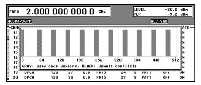
The code channels are equally distributed over the code domain
