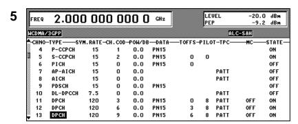
By going into the corresponding base station (BS 1 in this case) the channel table can be seen and parameters can be edited
