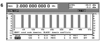
Press the STATUS – key on the SMIQ front panel: the code domain is displayed
